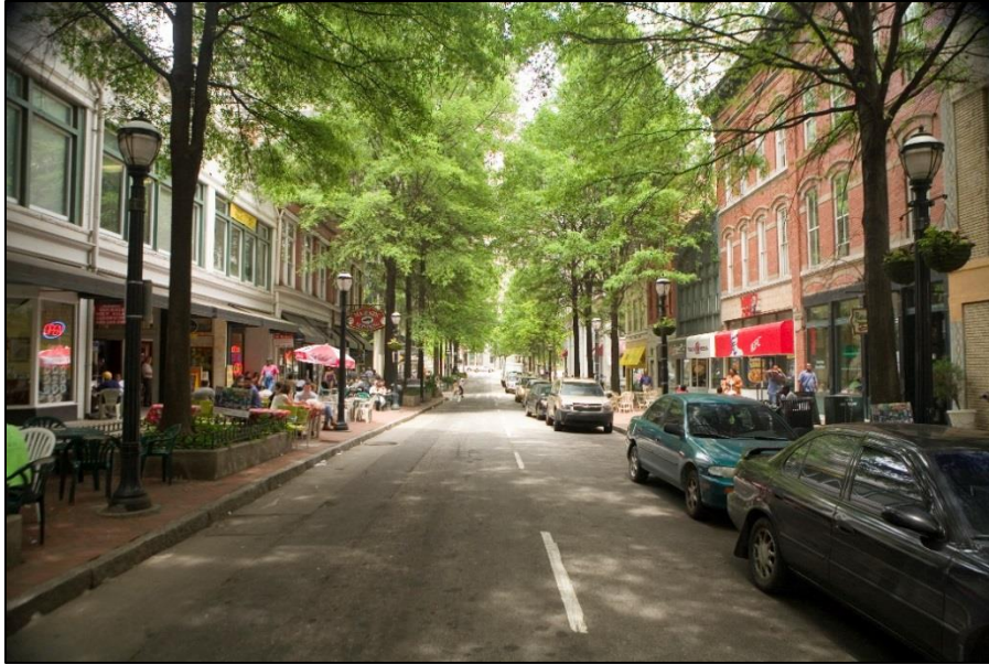
Figure 4.13. Roads are an important part of mixed-use developments. This development along 15th Street in Atlanta, Georgia, has narrower roads to provide room for wider sidewalks that improve walkability.
