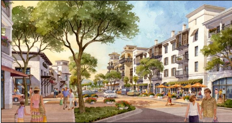
Figure 4.6. Each mixed-use development has a maximum height restriction. There are techniques for reducing the perceived height of an architectural structure. Using variations in colors, textures, and materials, will help visually break up the perceived scale of a building. Introducing street trees, awnings, benches, seating areas, and other street furnishings also helps create a pedestrian scale and reduces the visual impact of structures.
